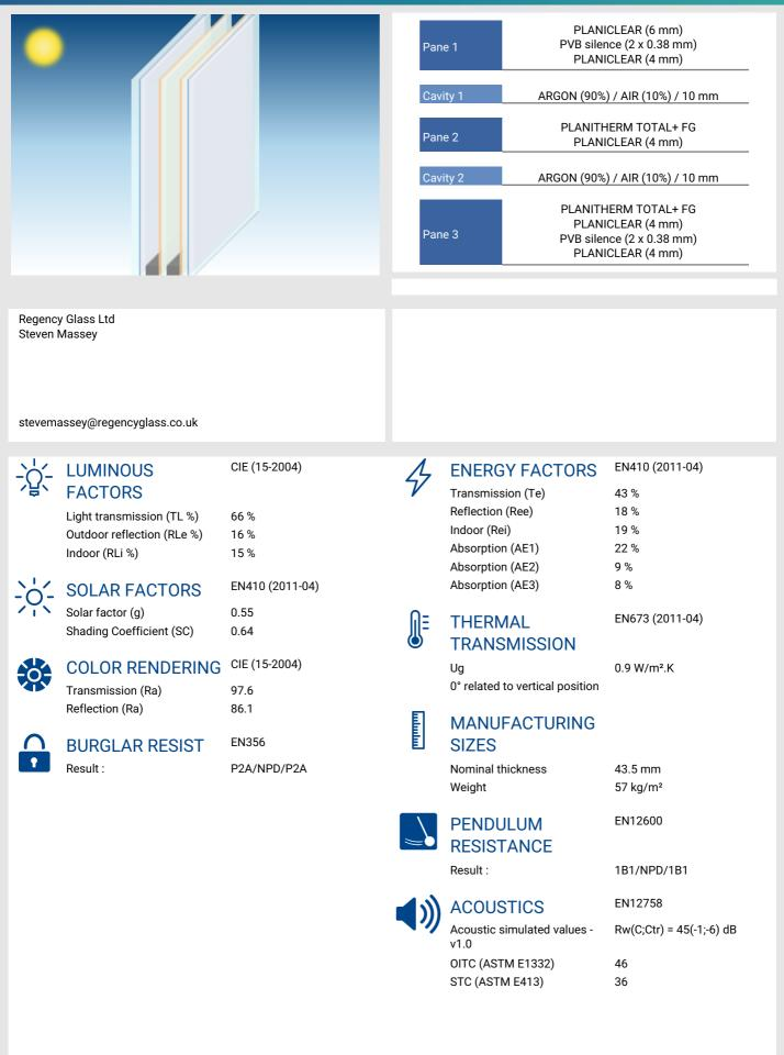
Result EN 410 EN 673 The sound attenuation indices are measured under laboratory conditions according to the standards EN ISO 10140 and EN 12758. The calculated indices are provided for information only. The accuracy for Rw index lies within a range of +/-2dB.The glass thickness calculations comply with the 2012 version of the DTU39-P4 description. The USER is responsible for ensuring that the correct calculation hypotheses are
