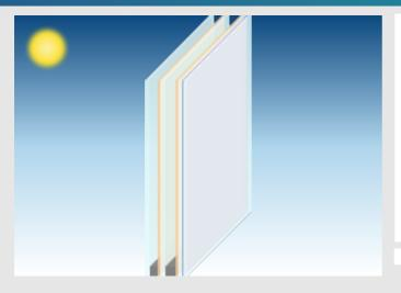
Pane 1 PLANICLEAR (4 mm) Cavity 1 ARGON (90%) / AIR (10%) / 6 mm PLANITHERM TOTAL+ FG Pane 2 PLANICLEAR (4 mm) Cavity 2 ARGON (90%) / AIR (10%) / 8 mm PLANITHERM TOTAL+ FG PLANICLEAR (3 mm) Pane 3 PVB silence (2 x 0.38 mm) PLANICLEAR (3 mm)
