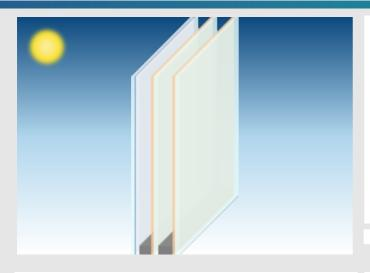
PLANICLEAR (3 mm) PVB silence (2 x 0.38 mm) Pane 1 PLANICLEAR (3 mm) KRYPTON (90%) / AIR (10%) / 10 mm PLANITHERM ONE T FG Pane 2 PLANICLEAR (4 mm) Cavity 2 KRYPTON (90%) / AIR (10%) / 12 mm PLANITHERM ONE T FG Pane 3 PLANICLEAR (4 mm)
