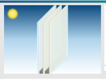
PLANICLEAR (3 mm) PVB standard (2 x 0.38 mm) Pane 1 PLANICLEAR (3 mm) KRYPTON (90%) / AIR (10%) / 10 mm Cavity 1 PLANITHERM ONE T FG Pane 2 PLANICLEAR (4 mm) Cavity 2 KRYPTON (90%) / AIR (10%) / 12 mm PLANITHERM ONE T FG Pane 3 PLANICLEAR (4 mm)
