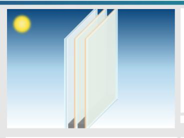
PLANICLEAR (3 mm) PVB standard (2 x 0.38 mm) Pane 1 PLANICLEAR (3 mm) ARGON (90%) / AIR (10%) / 10 mm PLANITHERM ONE T FG Pane 2 PLANICLEAR (4 mm) Cavity 2 ARGON (90%) / AIR (10%) / 12 mm PLANITHERM ONE T FG Pane 3 PLANICLEAR (4 mm)
