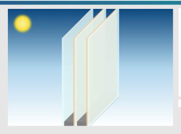
Pane 1 PLANICLEAR (4 mm) Cavity 1 ARGON (90%) / AIR (10%) / 16 mm PLANITHERM TOTAL+ FG Pane 2 PLANICLEAR (4 mm) Cavity 2 ARGON (90%) / AIR (10%) / 16 mm PLANITHERM TOTAL+ FG Pane 3 PLANICLEAR (4 mm)
