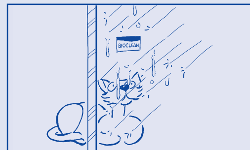
Always glaze the SGG BIOCLEAN face towards the exterior.
