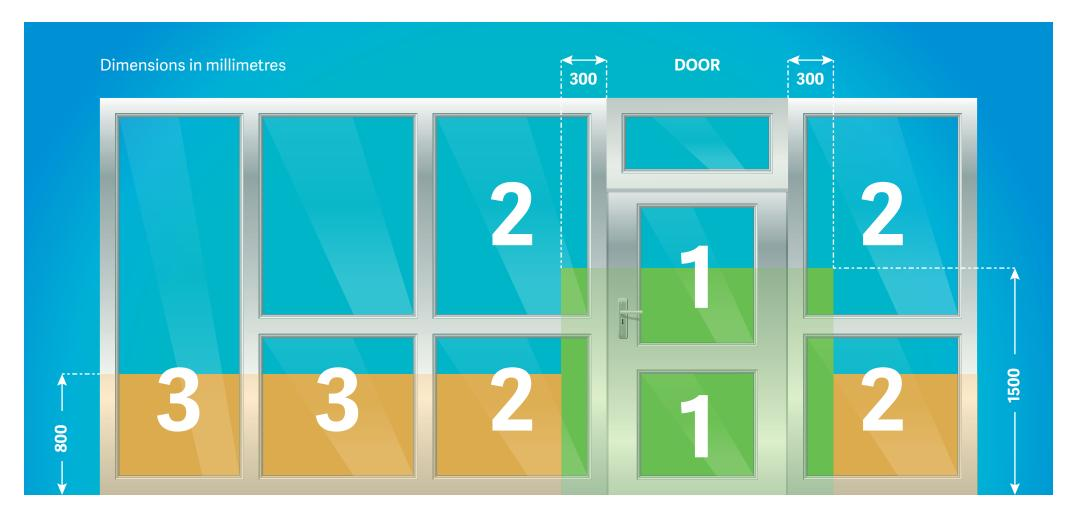
**Doors** (glazing wholly, or partly, within 1500mm from floor or ground level)
